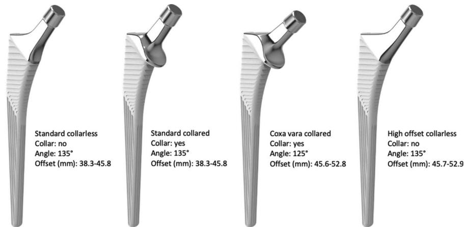
**Fig. 1.** The Corail® stem variants (DePuy Synthes) included in this study. From the left, the standard collarless, standard collared, coxa vara collared, and high offset collarless stems. Published with permission from DePuy Synthes.
