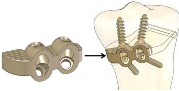
**Fig. 1** The iBalance medial opening wedge HTO system
