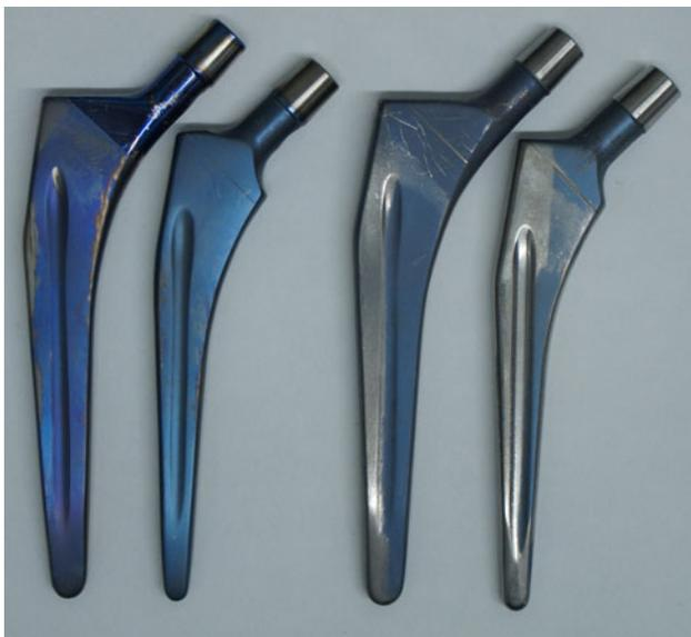
**Fig. 4** Retrieved Titan® stems show variations in proximal stem geometry and color between groups. Stems shown from left to right are Group A lateralized, Group A standard, Group C lateralized, and Group C standard.
