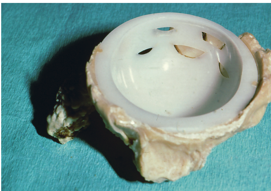
Figure 5 A Christiansen prosthesis revised at the Coastal Hospital in Hagevik. The Delrin cup has been worn right through. This cup (without the cement) was used by Leif Ivar Havelin and collaborators as an illustration of the wear in Christiansen prostheses (25). Such asymmetric wear on the cup is also a recurring feature of the Christiansen prosthesis depicted in the Norwegian Arthroplasty Register's logo. Photo: Einar Sudmann
