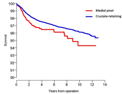
Fig. 2 This graph shows survival functions of the medial pivot and cruciate-retaining designs in Australia. Curves end when 20 patients are left at risk.
