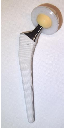
Figure 21. Marathon cup, Biolox forte head and Corail stem.
